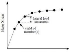
Roof Displacement Figure 1. Capacity (Pushover) Curve of Structure
