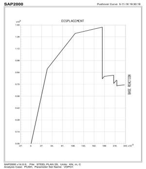
FIGURE 4. PUSHOVER CURVE OF 2 STOREY FRAME
