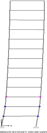
Figure 9. Immediate occupancy and Life safety level for 13  $$\operatorname{storeys}$
