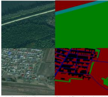
Fig .4. Satellite Images Classification by U-Net
